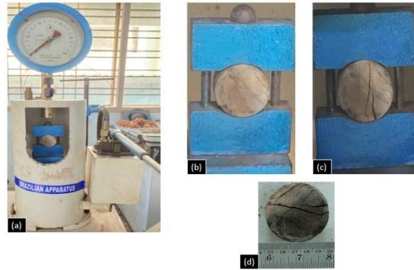
**Figure 2: Experimental setup for Brazilian tensile strength test (a) Brazilian apparatus to conduct the test (b) Rock specimen before the failure (c) Crack propagation under tensile loading (d) Rock specimen after the failure**
